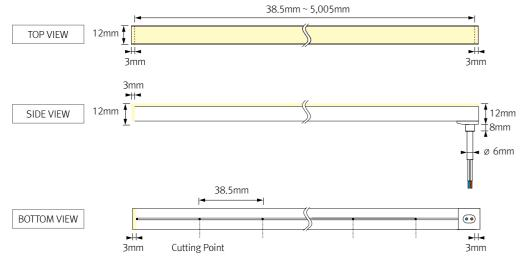
FLXible Neon can be cut every 38.5mm. Please follow the cutting point mark to cut precisely as needed.
